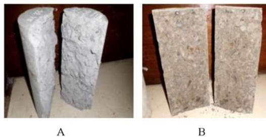
Figure 7 Cylinder concrete of organic cement (A). Cylinder concrete of portland cement (B)
