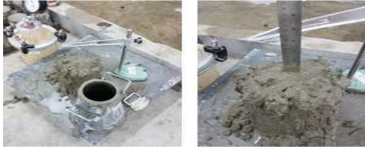
Figure 3 Slump test of fresh concrete organic cement
