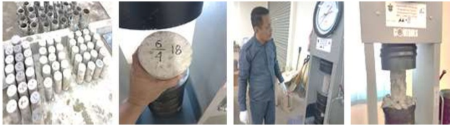
Figure 4 Test process of compressive strength cylinder concrete organic cement
